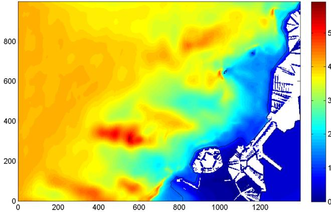
Fig. 17: Significant wave height for the simulation ( $H_{m0}=4m$ ,  $T_p=14s$ ,  $\theta=270^\circ N$  and a low tide water level of 1.45m)
