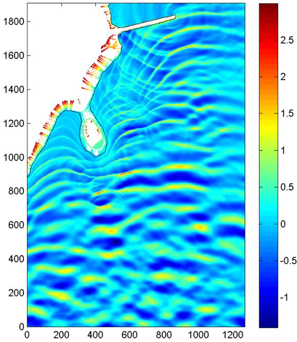
Fig. 11: Water surface elevation for the simulation at low tide ( $H_{m0}=2m$ ,  $T_p=12s$ , wave direction  $\theta=200^\circ N$  and a low tide water level of 1.45m)
