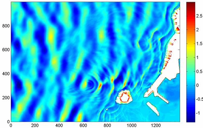
Fig. 13: Water surface elevation for the reference simulation (at  $t=40$ min,  $H_{m0}=2m$ ,  $T_p=12$  s,  $\theta=270^\circ$  and a mid-tide water level of 3.07m)
