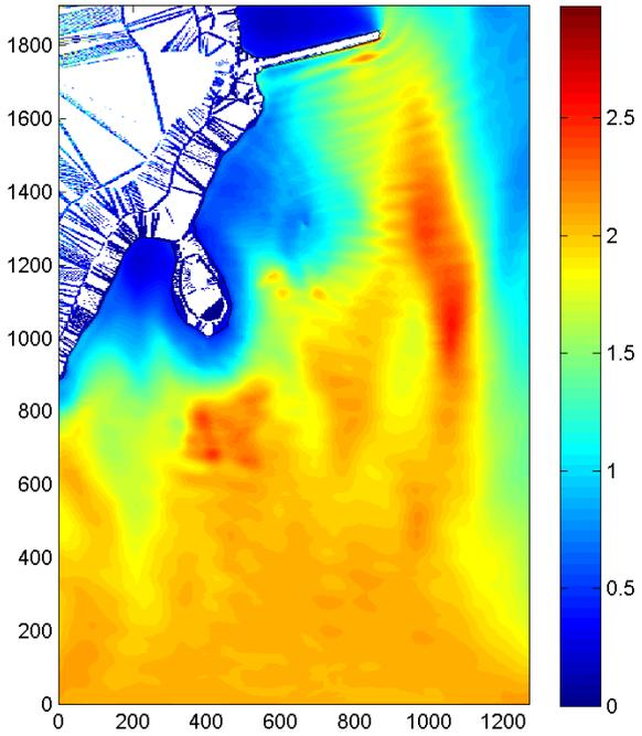
Fig. 12: Significant wave height for the simulation at low tide ( $H_{m0}=2m$ ,  $T_p=12s$ , wave direction  $\theta=200^\circ N$  and a low tide water level of 1.45m)
