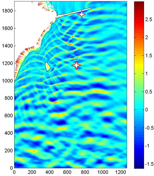
Fig. 6: Water surface elevation for the reference simulation ( $H_{m0}=2\text{m}$ ,  $T_p=12\text{s}$ , wave direction  $\theta=200^\circ\text{N}$  and a high tide water level of  $4.75\text{m}$ )
