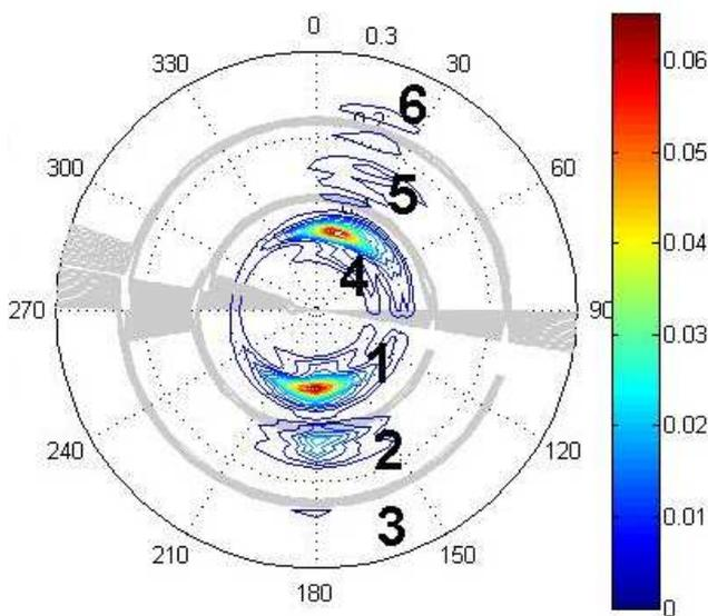
Fig. 10: Results of partitioning at point 1 for a 2m incoming Hm0 at high tide
