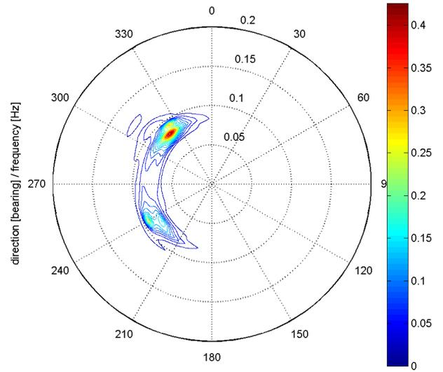
Fig. 15: Modeled directional spectra at point 7 with DIWASP (see Fig. 5) for the reference simulation
