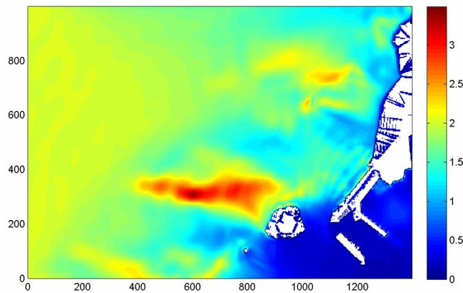
Fig. 14: Significant wave height for the reference simulation (mid-tide level)
